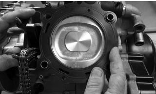
8. Install the four cylinder head cap screws with washers. Tighten only until snug.
