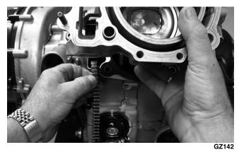
4. Loosely install the two nuts securing the cylinder to the crankcase.
