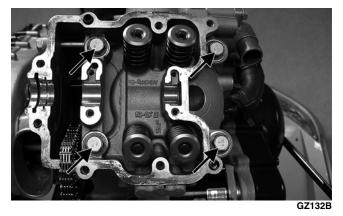
9. Loosely install the five cylinder head nuts.
