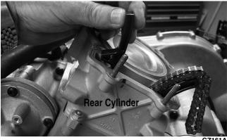
7. Place the head gasket into position on the cylinder. Place the alignment pins into position; then place the head assembly into position on the cylinder while guiding the cam chain through the cylinder head.
